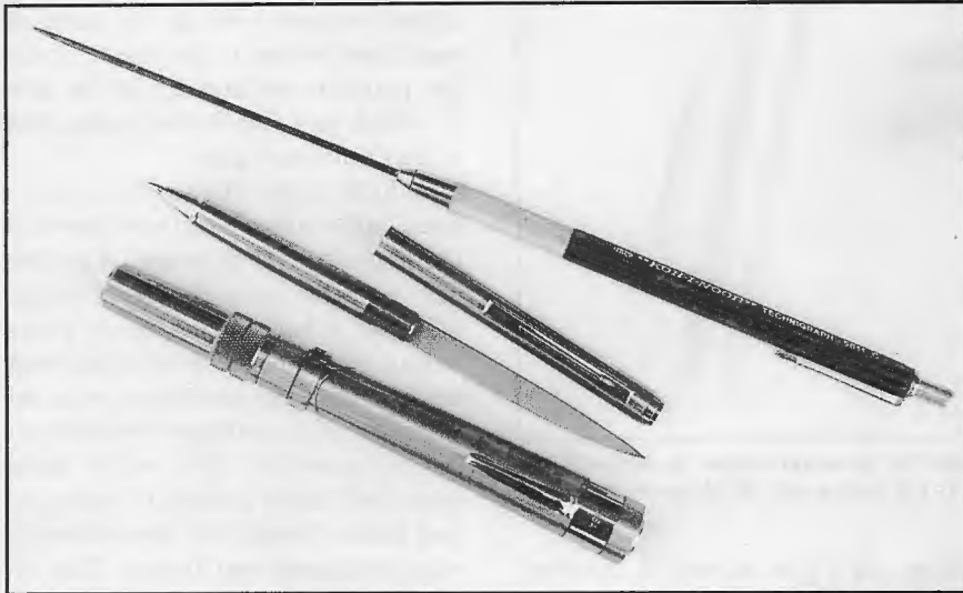
An assortment of deadly lapel-pocket devices, from top to bottom: rod pencil, a specially modified KOH-I-NOR drafting pencil with a spring-loaded 3.3-inch hardened steel shaft that tapers to a needle point; a dagger within a ballpoint pen; and the Stinger Pen Pistol in its pen configuration.
